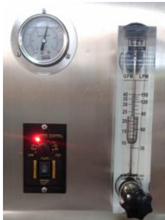
Pressure gauge & Flow meter
